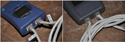
Example of indication by the tester with an interrupted a pair of 7-8:
