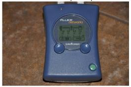
Example, indicate the case when which the wires in a pair of 7-8 are swapped:
